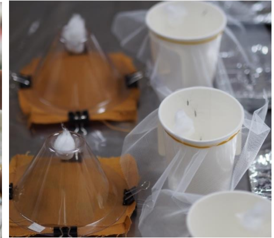
Right: Performing WHO cone tests on patches of worn ITC/NTC
